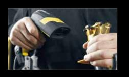
By scanning the tool identification codes on the presetting and measuring machine, the tool data is called up directly and the measuring process can start.
