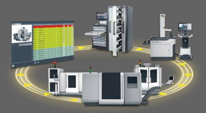
The »flash« production analysis software communicates directly with the CNC machine and gathers the current tool life. Their status is pointed out in red, yellow, and green on the monitor. This allows you to make the best possible use of the tool life while maintaining the same process reliability. At the same time, timely tool preparation minimizes waiting times at the machine and leads to an efficient production workflow.
