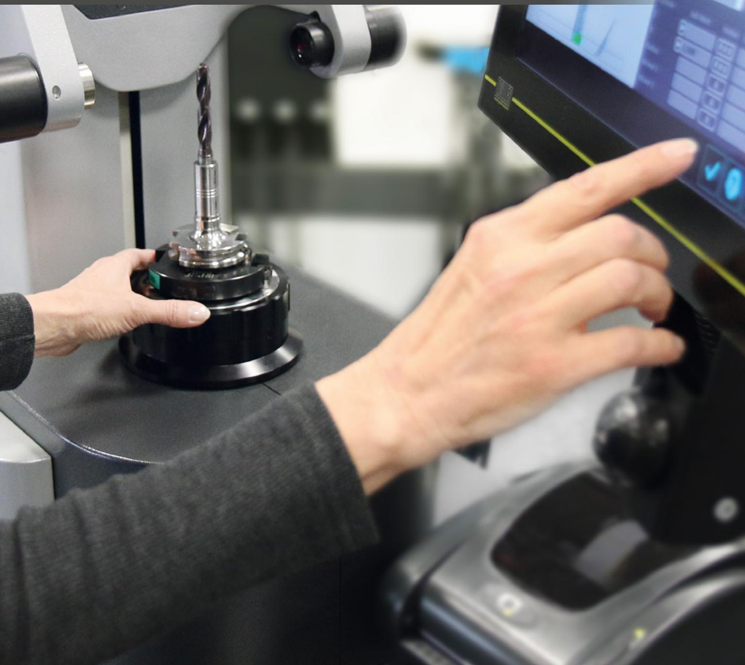
The new image processing technology »pilot 1.0« offers all functions for presetting and measuring standard tools quickly and easily. For instance „Automatic cutter shape and measuring range detection“,
