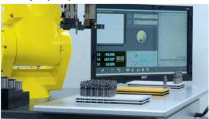
Using a 'pallet administration' facility incorporated in ZOLLER's »pilot 3.0« software, loading configuration and parameters are defined. That means that all tools can be measured without further user input, and customerspecific pallets can be defined.
