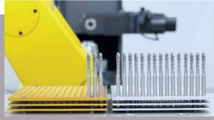
On completion of the measuring process, defective tools have already been sorted out from the good tools. Measuring values for the individual tools are stored in »pilot 3.0« and can be sourced and issued when required.
